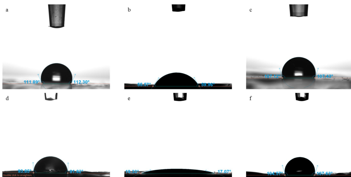
Figure 2. Contact angle of (a) gelatin based film, (b) HPMC based film, (c) pectin based film, (d) HPMC-gelatin based film, (e) pectin-HPMC based film, and (f) pectin-gelatin film.
