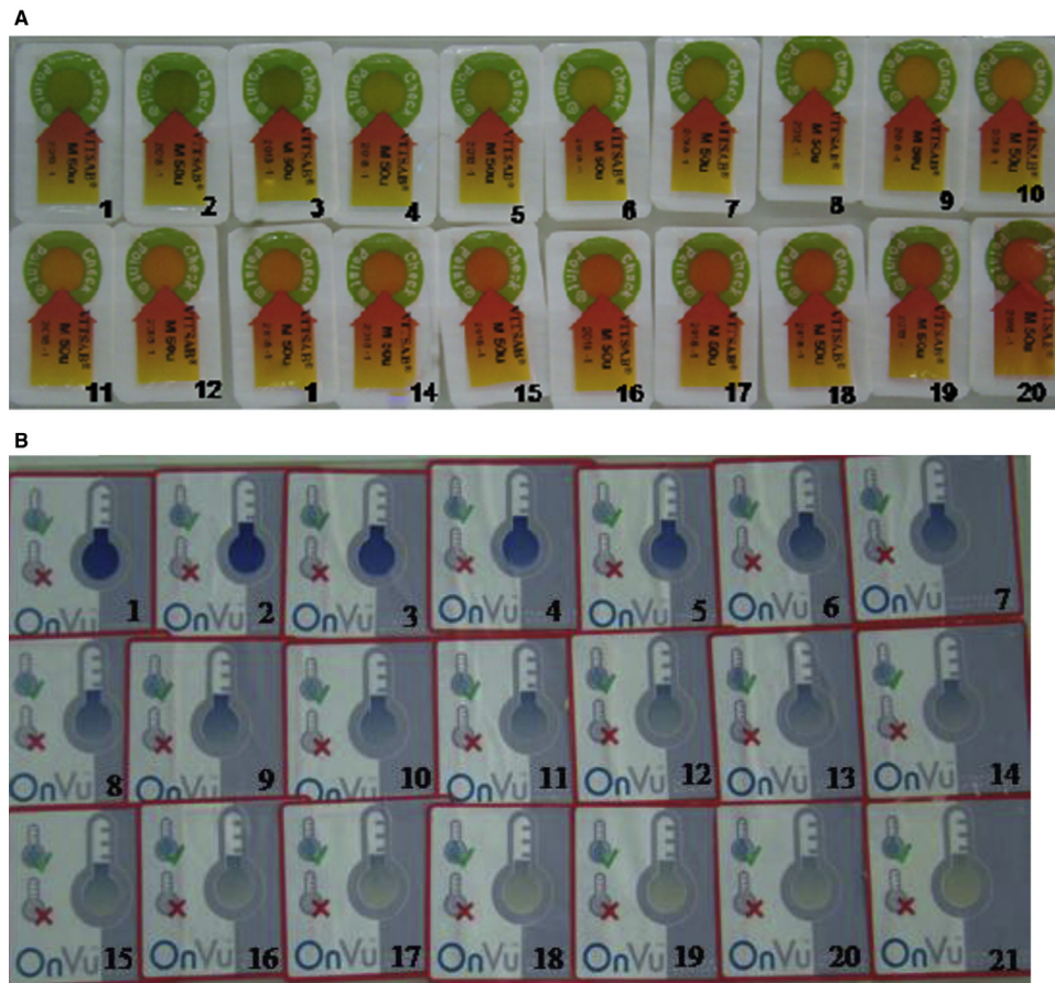
Figure 9 (A) M-type enzymatic TTI label color scale, (B) OnVu™ TTI photochromic TTI label color scale.
