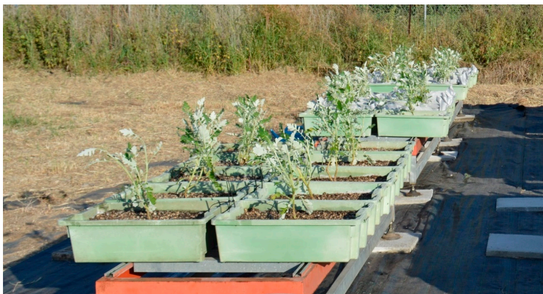
Figure 1. Experimental setup of the simulated extensive green roof modules with Jacobaea maritima subsp. sicula plants at the experimental field of the Laboratory of Floriculture and Landscape Architecture, Agricultural University of Athens.
